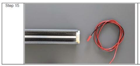
Pull battery cable out of HeadRail XL20.
